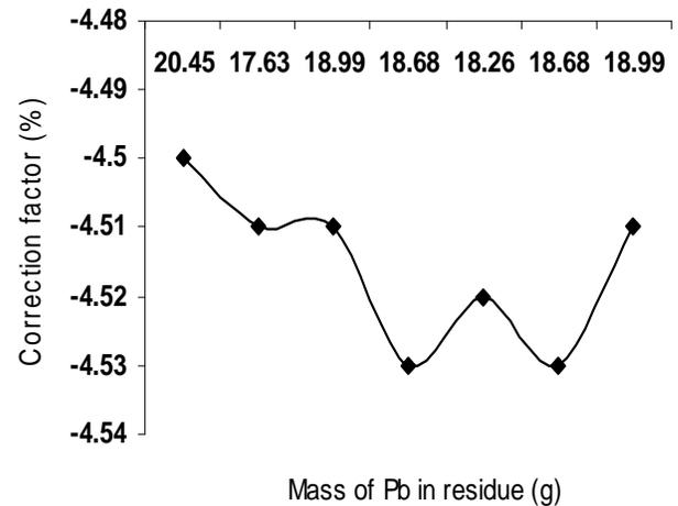
**Figure 3: Variation of model-predicted mass of lead (in residue) with its associated correction factor**
