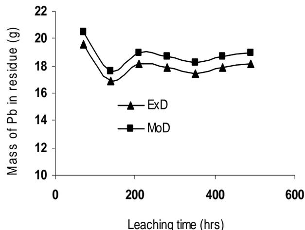
**Figure 1: Comparison of the masses of lead (sipping into the reaction residue) as obtained from experiment [6] and derived model.**
