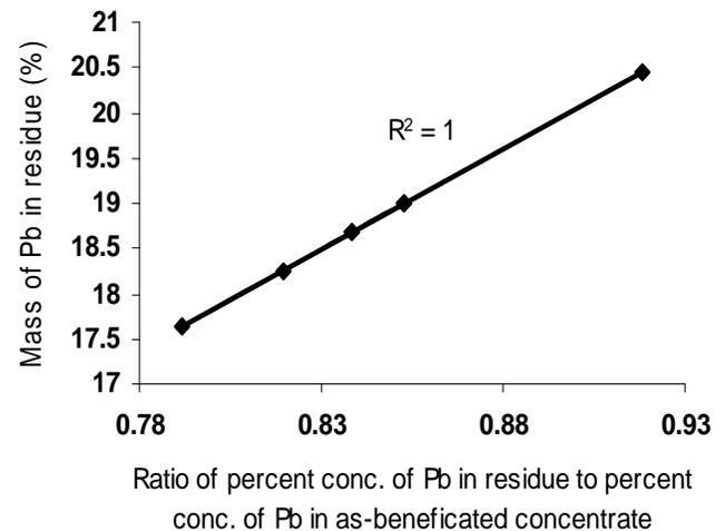
**Figure 4: Variation of  $\beta_R / \beta_i$  ratio with model-predicted mass of lead in residue**
