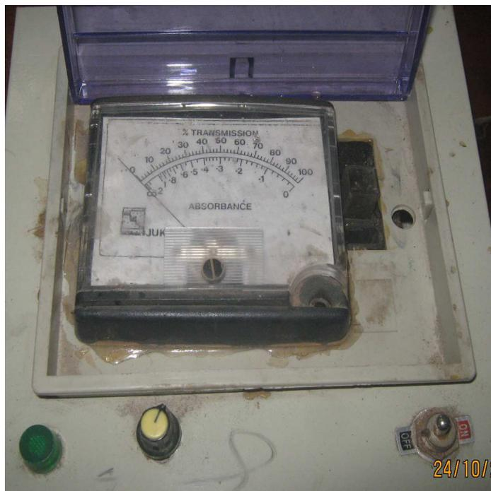
Figure 1: The Locally fabricated Colorimeter
