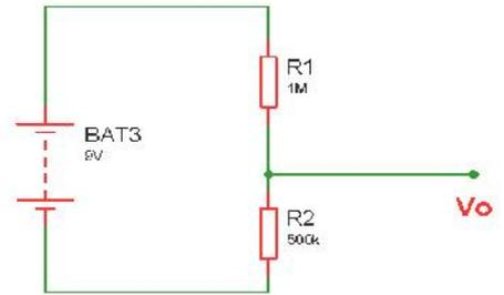
**Figure 3: A voltage divider circuit**
