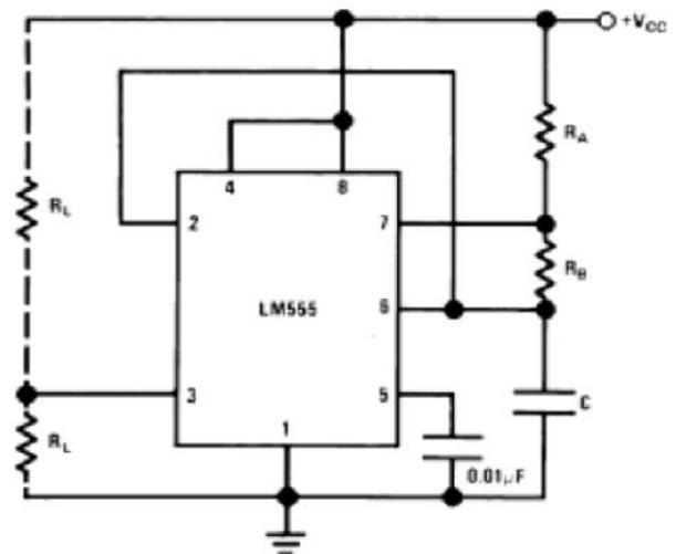
Figure 8: LM555 as an astable multivibrator (Jameco,
