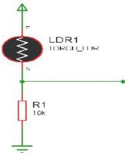
**Figure 9: The LDR as a voltage divider**
