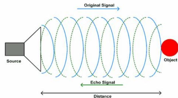
Figure 1: The working principle of Ultrasound (ElectronicWings, 2019)
