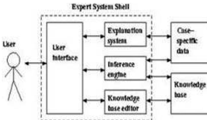
Figure 2: The Structure of the Expert System
