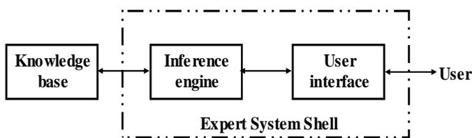
Figure 1: The Simplest form of an Expert System
